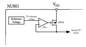
When the  $V_{DD}$  power is under 5V, the OPA will drive the PMOS to fully turn on state. Due to the variation of the chip fabrication process, the driving capability of PMOS and OPA will also vary and decrease in different chips. That will prolong the establishing of internal power of chip when  $V_{DD}$  is under 5V. The delay time will be longer if the capacitor connected to V5 pin of NU801 is larger. The recommended capacitance is listed in the following table.
